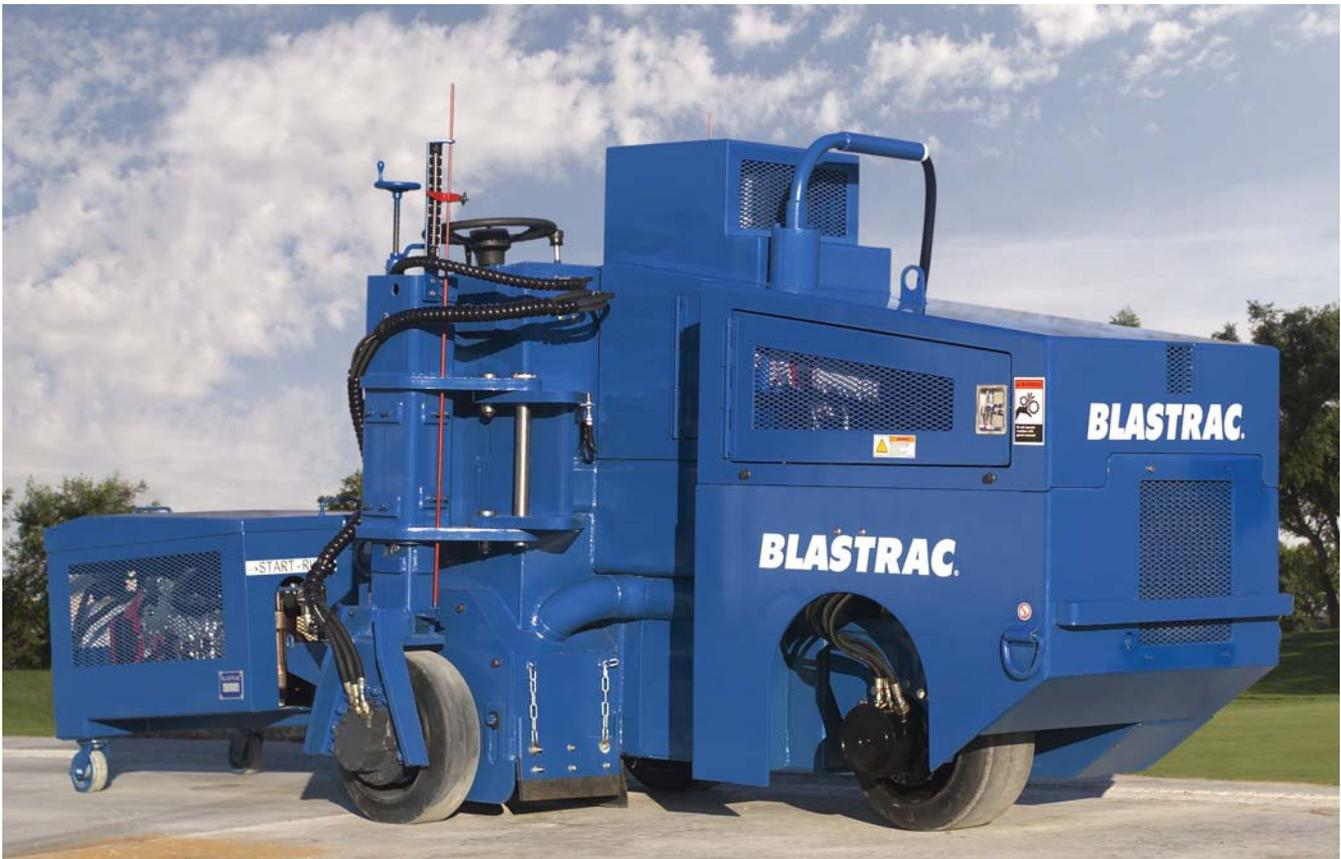
The Blastrac® BMP 6000 electric milling machine is designed for heavy surface preparation. Different milling cutter configurations allow this machine to remove concrete, overlays, asphalt, troweled down epoxies, elastomeric coatings, thin-set mortar, grout beds, and flooring materials such as ceramic tile.
